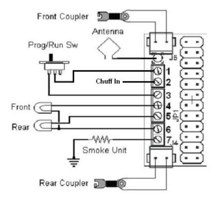
Note: There are two (2) commons on the card marked "com" on pins 3 and 6. These are electrically the same. Do NOT return the smoke unit common to the Cruise commander; attach to the chassis instead. When the feature pin (7) is a strobe or cab light, the return on these may be attached to pin 6 (or 3).
